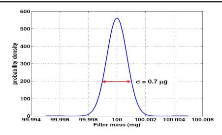
The uncertainty of PM loading on the filter is twice the variance of the repeatability of the filter measurement.
