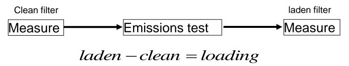
Multiple measurements of each filter paper before and after PM loading is statistically beneficial but time consuming.
