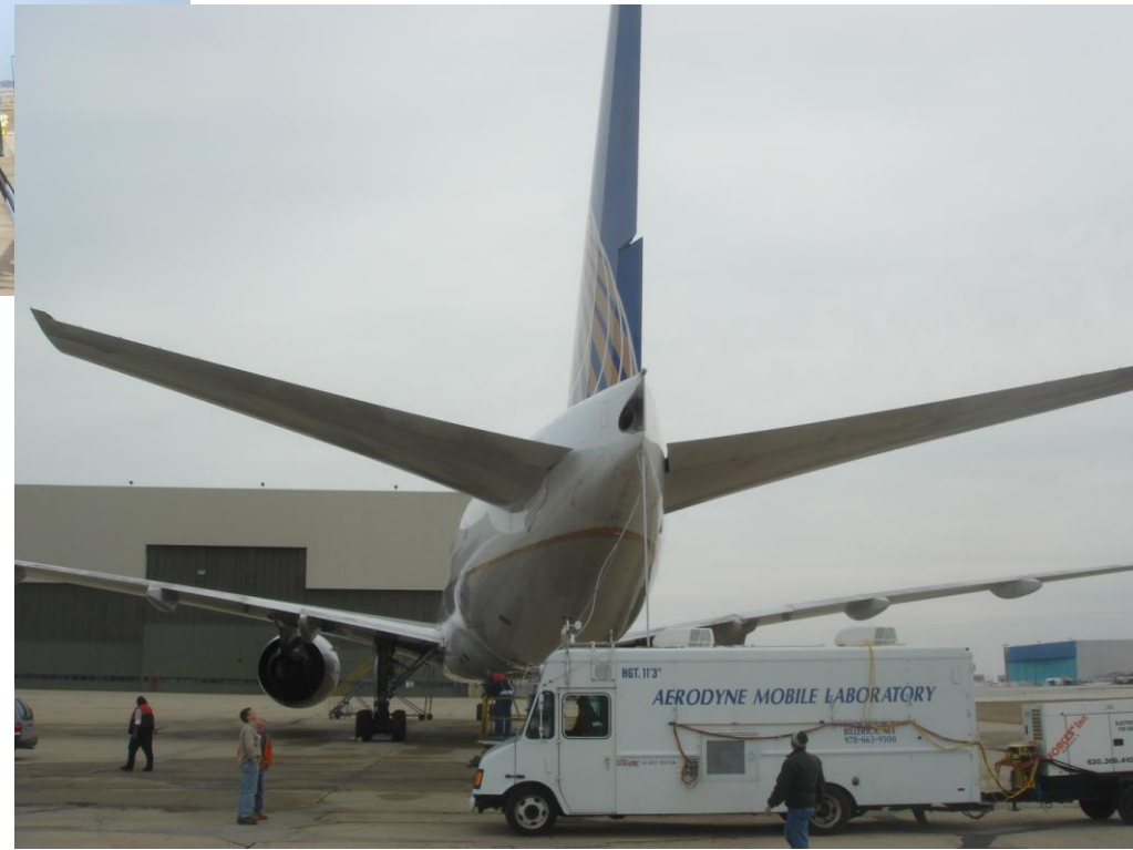
B777 aircraft with GTCP 331-500 APU
