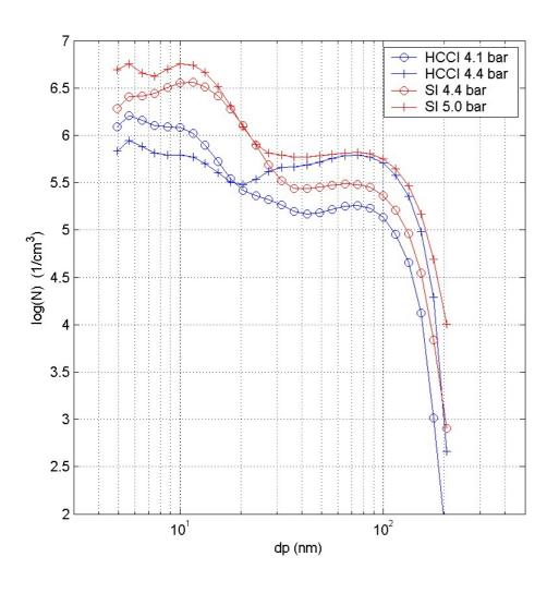
At the same load (4.4 bar), the # concentration of the acc' mode from HCCI is a factor of  $\sim 3^* >$  than from SI
