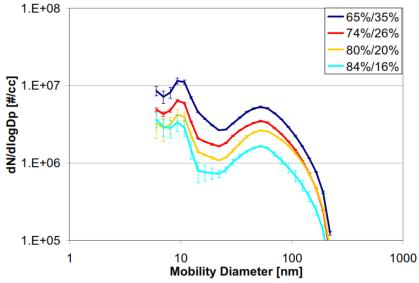
Figure 1: Particle Size Distribution Measurements from 65%-35% to 84%-16% Gasoline-Diesel Proportioning at Fixed Gasoline and Diesel In-Cylinder Injection Timings.
