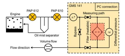
Figure 1: Schematic of the Topas/Adaptive oil blow-by measurement system.
